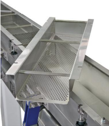
Using a vibrating sieve, the tobacco is separated from the paper and filters and returned directly to the hopper on the maker where it is mixed together with the new tobacco.
